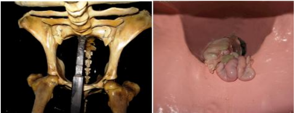
Figure 1: The Bovine Trans-Rectal Palpation Phantom has been designed with detailed inside structures of pelvis and was based on the anatomy of a dual-purpose Iranian-Holstein mixed breed.
